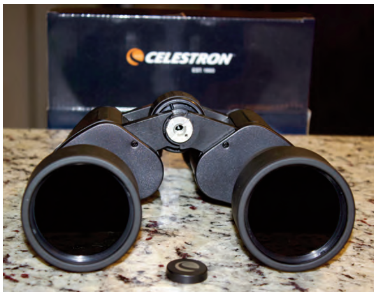
Image 19 - Tripod adaptable binoculars often have a 1/4-20 slot on the front side of the binocular bridge.
