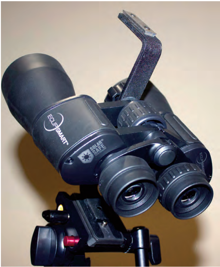
Image 21 - This view shows how the binocular Z bracket attaches to both the tripod and binoculars.
