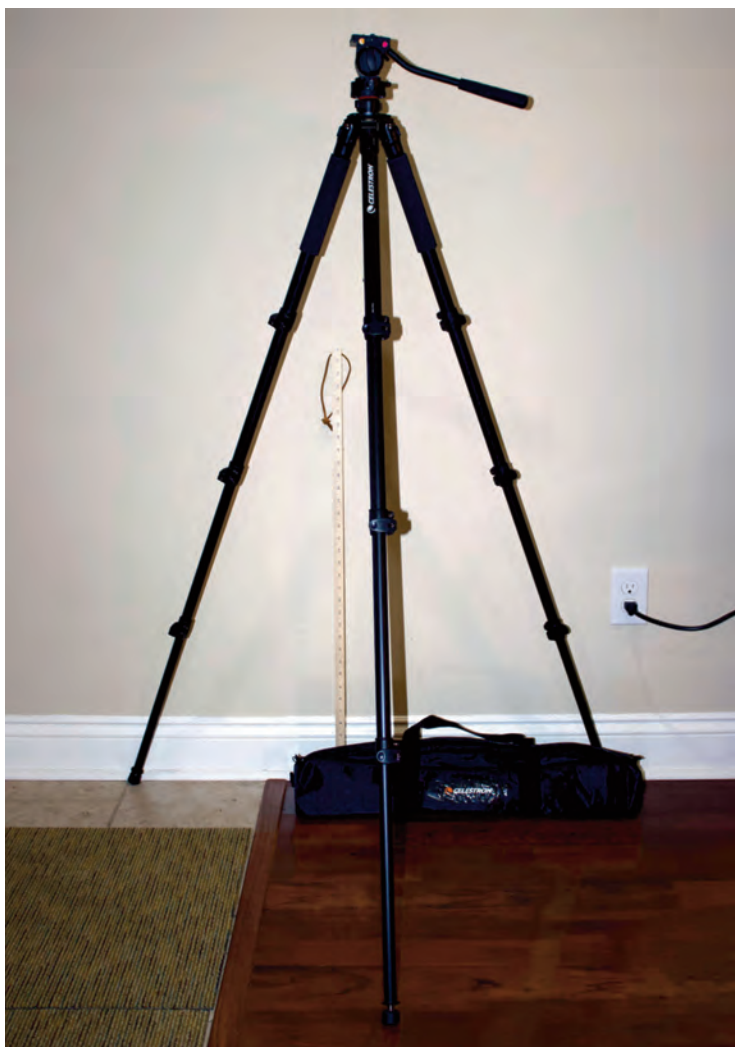
Image 15 - The Celestron Regal tripod with its soft case. The tripod is great for holding small binoculars that have a 1/4-20 threaded tripod slot.
